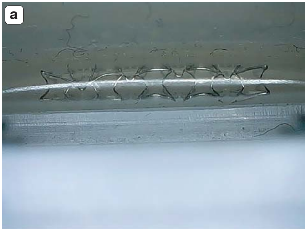
Fig. 2. Sample of the 1st stent before (a) and after (b) the deformation test.
