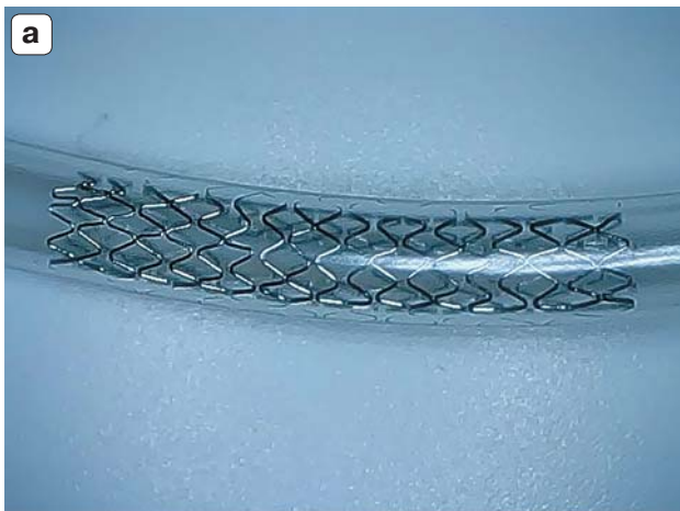
Fig. 3. Sample of the 2nd stent before (a) and after (b) the deformation test.
