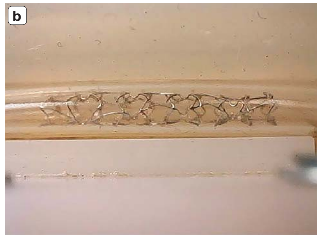
Fig. 2. Sample of the 1st stent before (a) and after (b) the deformation test.
